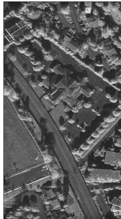
Figure 1 | Photographic-quality imagery is generated by the multimode Lynx Block 20A radar system from General Atomics Aeronautical Systems, Inc. (GA-ASI).
