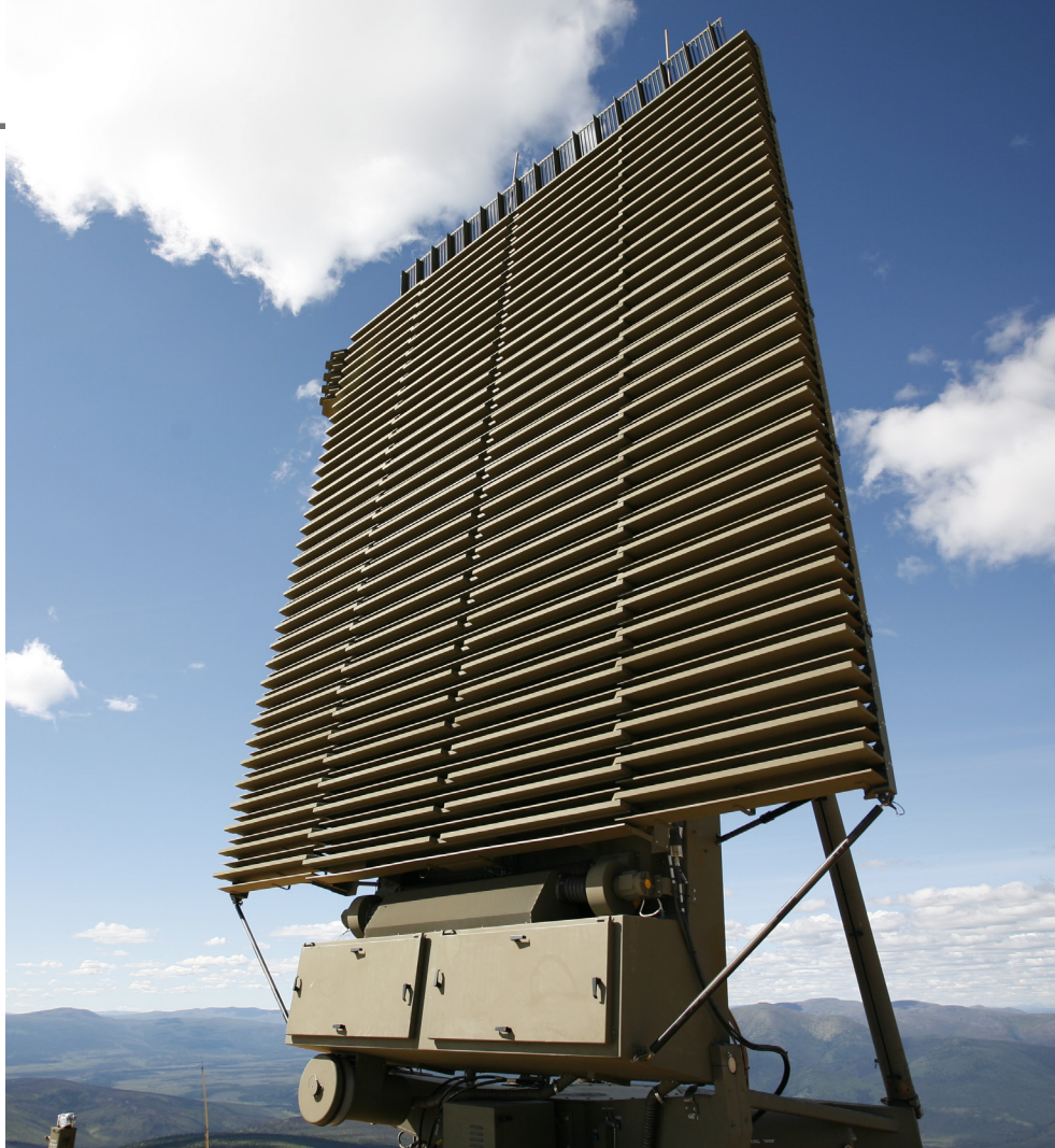
The TPS-77 portable long-range radar from Lockheed Martin Mission Systems & Training is mitigating, via sophisticated signal processing techniques, many of the false alarms caused by wind farms.
