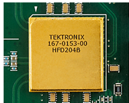
Figure 1 | Tektronix Component Solutions' SiGe-based ADC provides 12.5 GSps digitization performance to the TADF-4300 module.
